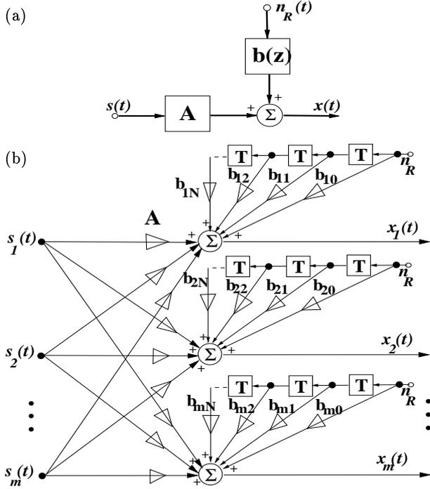
**Figure 1. The mixture and noise model: (a) source mixture with additive noise vector; (b) modeling the unknown noise by a convolutional additive noise ( $n_R$  is the reference noise, the  $b_{ij}$ -s are unknown).**
