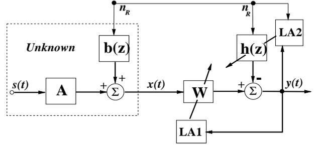
**Figure 2. The basic demixing model with two simultaneous learning steps ( $LA1, LA2$  means learning algorithms).**
