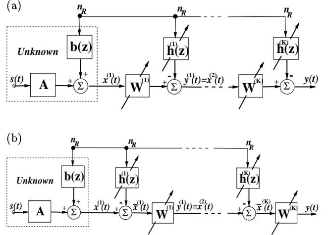
Figure 4. Alternative multi-layer neural network models for blind separation with noise cancellation.
