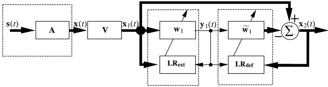
Figure 1: Functional block diagram of the 1st extraction single neuron and the 1st deflation network.  $\mathbf{LR}_{\text{ext}}$  and  $\mathbf{LR}_{\text{def}}$  stand for the extraction learning rule and the deflation learning rule, respectively.
