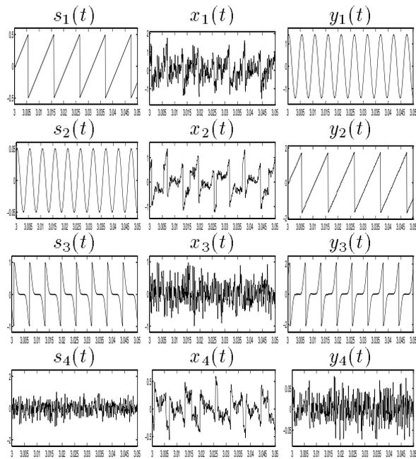
Figure 1: A typical result of extraction of four sources (with 10 KHz sampling rate), where  $s_k$ ,  $x_k$ , and  $y_k$  stand for the  $k$ -th source, mixed, and extracted signals, respectively.
