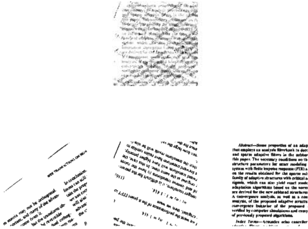
Fig. 2 Blind separation for one mixture of three text sources in Example 2. The first row: available image corrupted by other texts, the second row: three reconstructed texts.
